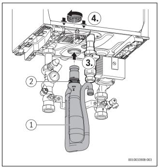
Fig. 16 Mounting the boiler siphon
