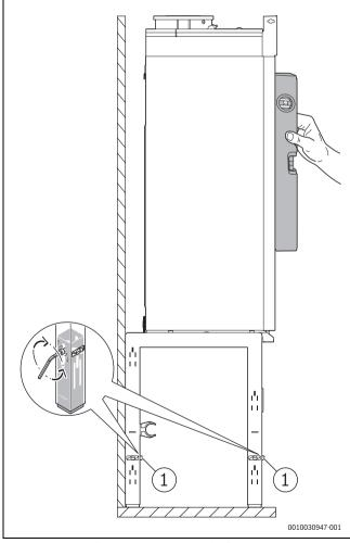
Fig. 10 Align the floor standing boiler on the frame
