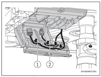
Fig. 26 Connecting the pump
