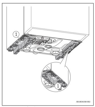
Fig. 7 Position of handle recesses
