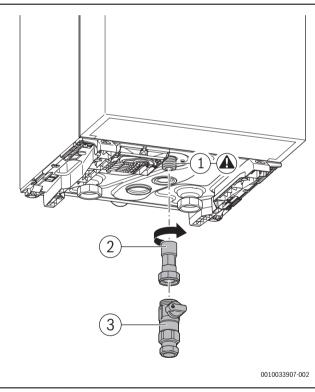
Fig. 13 Installing the gas valve
