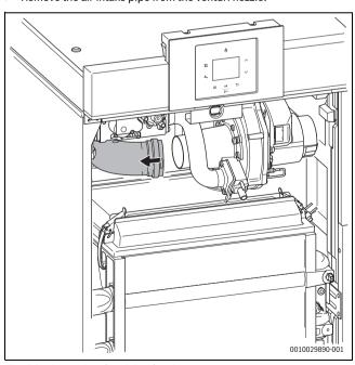
Fig. 36 Removing the air intake pipe
