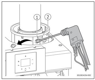
Fig. 32 Remove the plug on the flue outlet
