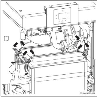
Fig. 37 Open the snap fasteners
