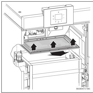
Fig. 40 Removing the burner
