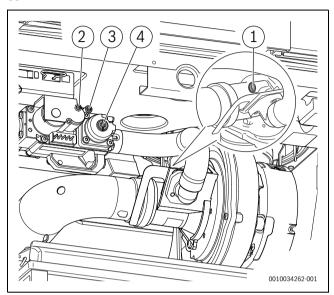
Fig. 30 Overview of test ports and adjusting screws ≤ 70 kW
