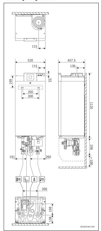
Fig. 3 Dimensions on the wall [mm]
