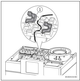
Fig. 24 Positioning the connecting lead and cable conduit
