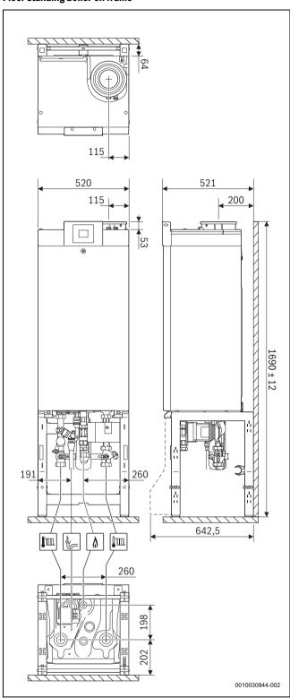
Fig. 2 Dimensions on base frame [mm]
