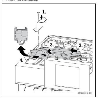
Fig. 47 Replacing the coding plug
