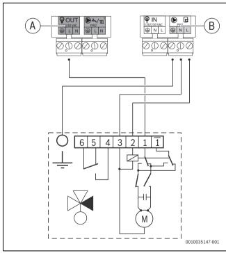
Fig. 27 Connection diagram for 230 V 3-way valve
