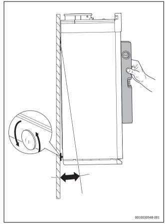
Fig. 12 Aligning the floor standing boiler on the wall
