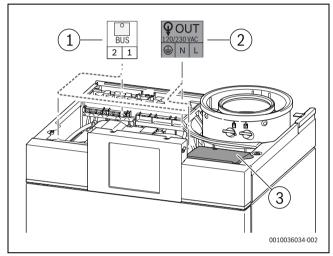
Fig. 28 Mounting the function module
