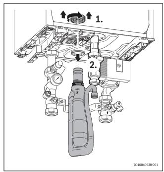
Fig. 42 Remove the boiler siphon
