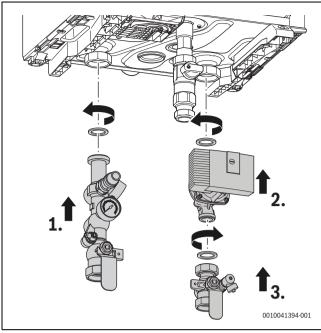
Fig. 14 Mount the flow/return connection
