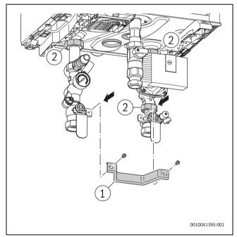
Fig. 15 Mount the brackets
