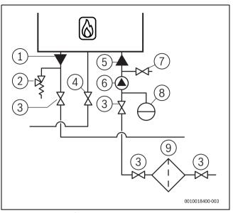
Fig. 18 Connection of heating water pipes
