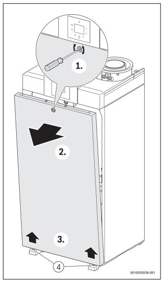
Fig. 6 Opening the front panel
