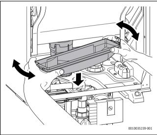
Fig. 44 Remove the condensation catch pan.
