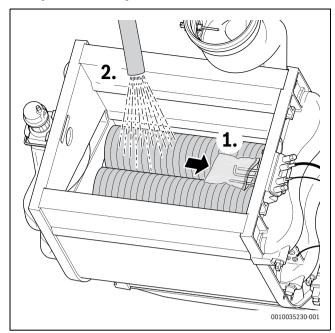
Fig. 41 Cleaning the heat exchanger
