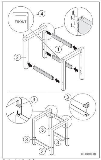
Fig. 8 Installing the frame
