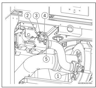
Fig. 31 Overview of test ports and adjusting screws ≥ 85 kW
