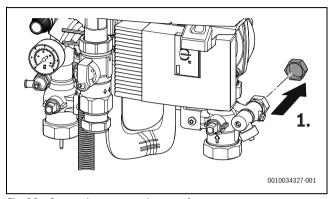
Fig. 20 Connecting an expansion vessel
