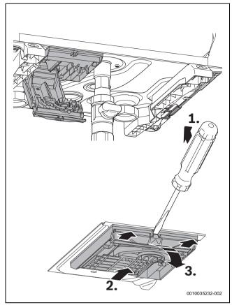
Fig. 25 Opening the pump terminal unit
