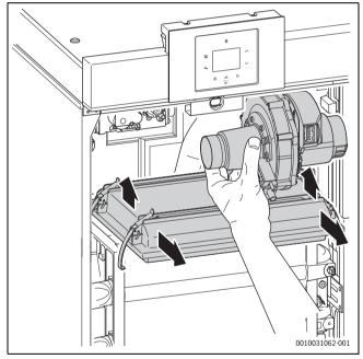
Fig. 38 Remove the gas-air unit together with the burner cover.
