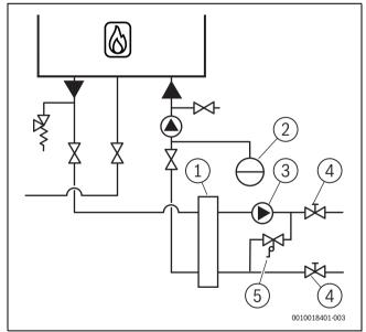
Fig. 19 Setup with low loss header
