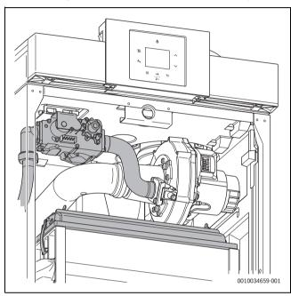
Fig. 33 Inspecting the gas path
