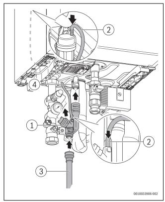
Fig. 17 Mounting the air vent valve hose
