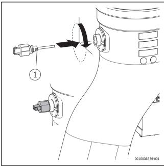
Fig. 46 Replacing the flue gas temperature sensor
