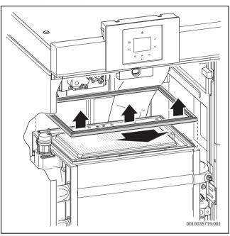
Fig. 39 Removing the burner gasket
