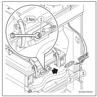
Fig. 45 Inserting the igniter
