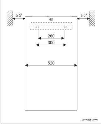
Fig. 5 Front view [mm]
