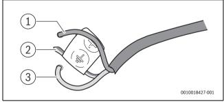
Fig. 29 Fitting the plug
