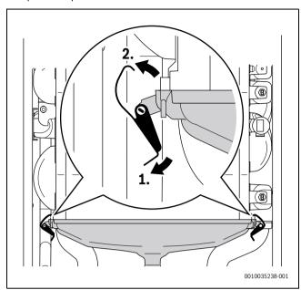
Fig. 43 Open the snap fasteners of the condensation catch pan
