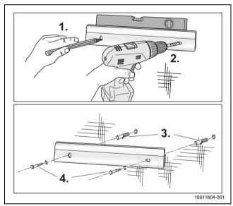
Fig. 11 Installing the mounting rail on a concrete wall
