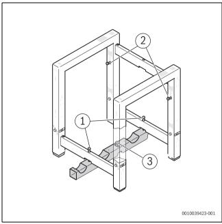
Fig. 9 Secure the frame to the wall or floor
